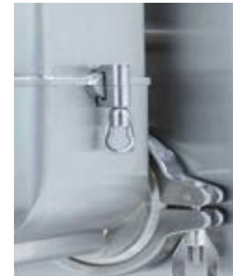
Quick-release fasteners for screws and screw tubes
