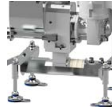
Rounded surface design for minimal particle deposition
